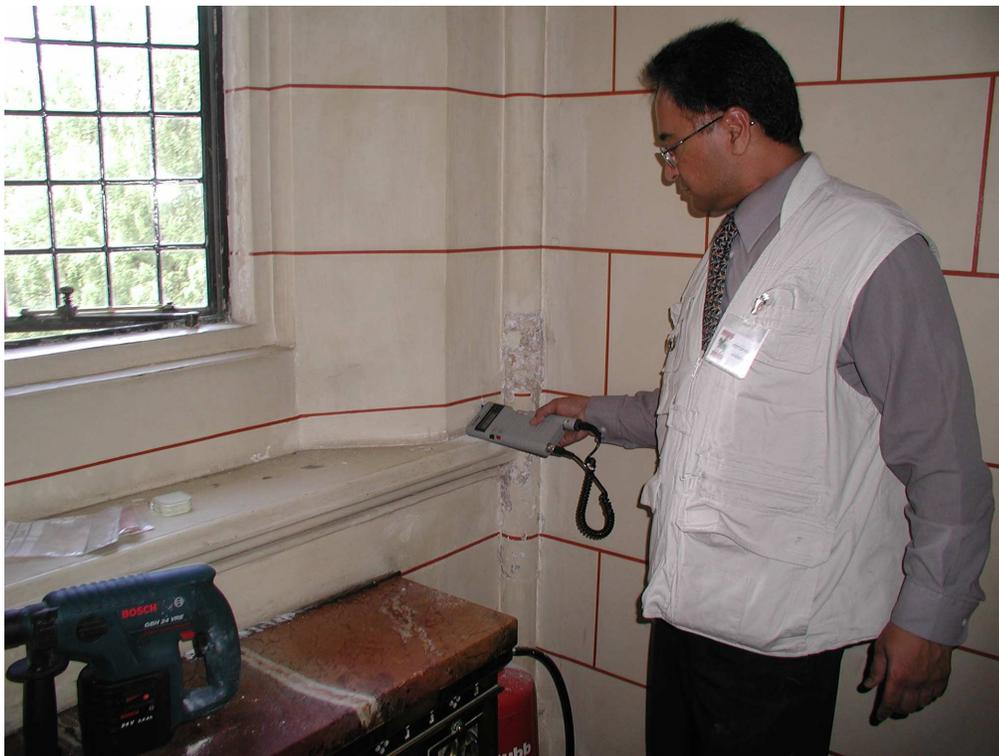
They can also be used to measure moisture contents of masonry but great care should be taken in interpretation of results as they are adversely affected by, certain paint finishes, salts and condensation. They are most useful in giving a measure of surface dryness. If high readings are identified then further investigation will be necessary possibly using mortar sampling if circumstance allow.
